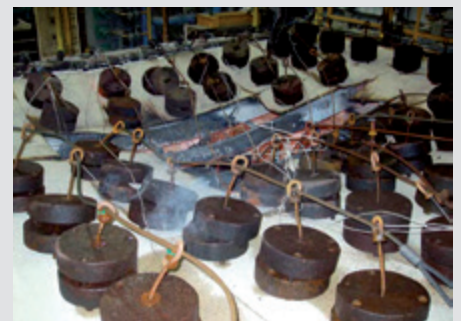
Light steel floor after a loaded fire test
