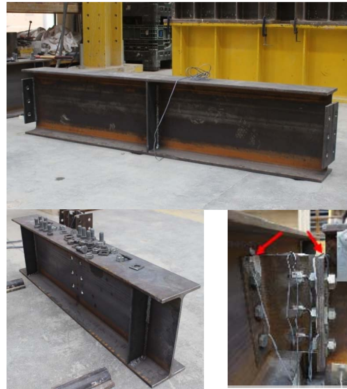
Dis-assembled steel components after tests and observed bolt slip during the first test
