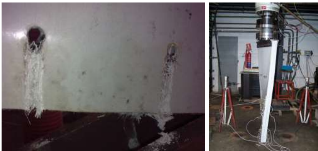
Figure 5. Load test to evaluate the capacity of bolted connections (left) and axial capacity of web panels (right).
